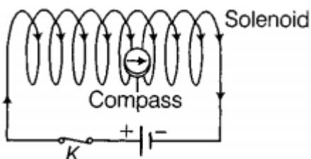
ii. The direction of the magnetic field inside the solenoid always points from the induced South pole towards the induced North pole.
